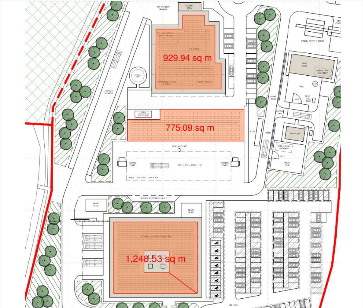
Figure 8: PV Array shown on the site plans on top of the BA block, Training Block as well as on external elements
